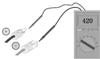
Figure 2-9 PV polarity check
